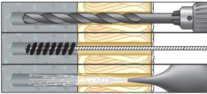
1. Drill a hole: Drill hole depth + insulation thickness
