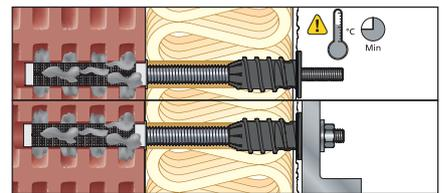
9. Observe curing time of the injection system, see cartridge label of the ResiFIX injection mortar.
