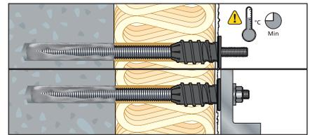
7. Observe curing time of the injection system, see cartridge label of the ResiFIX injection mortar.
