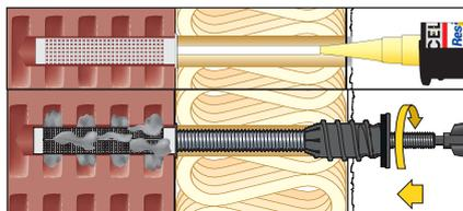
7. Fill the plastic sleeve completely with composite mortar (start from the beginning). For number of strokes see mounting instructions at [www.celofixings.com](http://www.celofixings.com)
