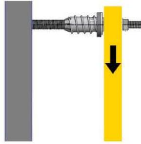
**Maximum shear loads  $V$ <sup>1)</sup> at max. 3 or 5 mm displacement per ResiTHERM®
