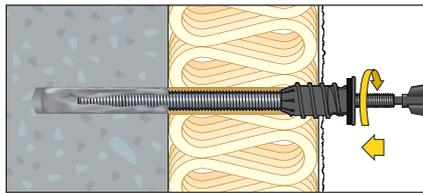
6. Screw in the ResiTHERM® 16 or 12 with the hexagon bit (included) and a cordless screwdriver until the seal is pressed against the plaster.
