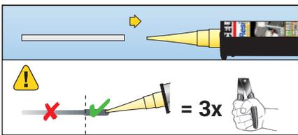
6. Attach the mixing nozzle extension MDV to the mixing nozzle MD.
