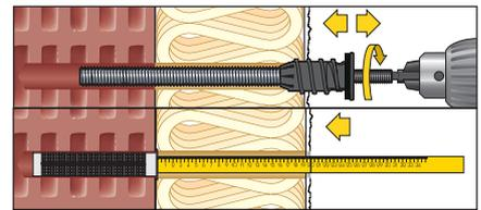
4. Enlarge the opening in the plaster for the collar of the plastic sleeve to 26 mm. To do this, briefly screw the thermal separation module in and out through the plaster for only approx. 2 thread turns or ream the plaster with a drill or drill with a bigger 26 mm drill.
