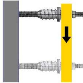
**Maximum shear loads V <sup>1)</sup> at max. 3 or 5 mm displacement per ResiTHERM<sup>®</sup> if the free outer end of the ResiTHERM<sup>®</sup> 16 & 12 is not freely rotatable (e.g. connected double fixing) at 24°C/40°C <sup>2)</sup>**
