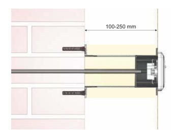
There is necessary to cut the carrier including inserted insulation before installation depending on layer thickness insulation.
